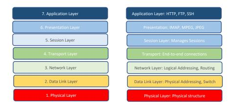
Here is a schematic diagram of the OSI model:
